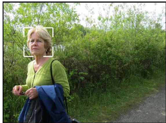
The ID box will become a green square when the release is partially depressed and focusing is acquired.
